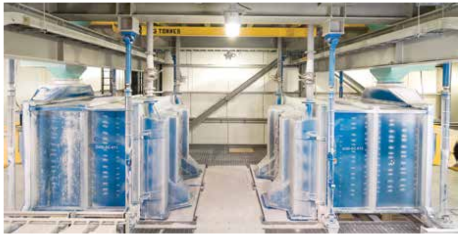
KSPC Fertilizer Product Loadout Area - Two Rotex mineral separator model MM5430-2 units.
