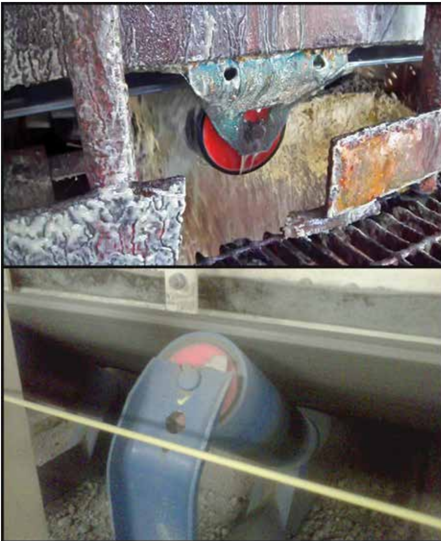
The HMS High Moisture Seals address two major causes of conveyor idler roller failure - jammed rollers and bearing contamination. The water from wash-down seen here was prevented from entering the roller ends, thus greatly extending the life of the operation's rollers.
